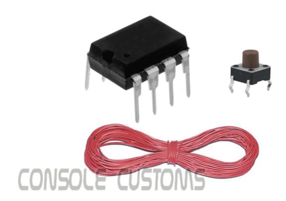
Step 1: You will start by taking the PIC chip and putting it on its back, also called (dead bug). Note the location of the notch that is on the top of the chip, the pin numbers and their purpose.
