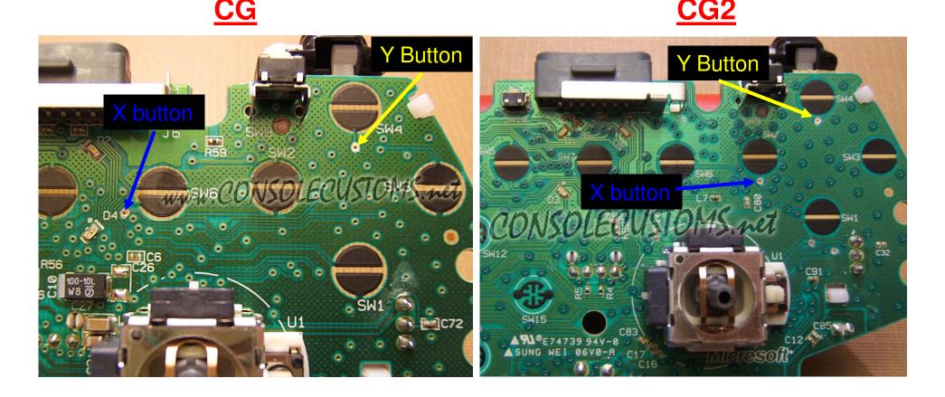
Step 6: Now we will attach the chip to the PCB using hot glue.
