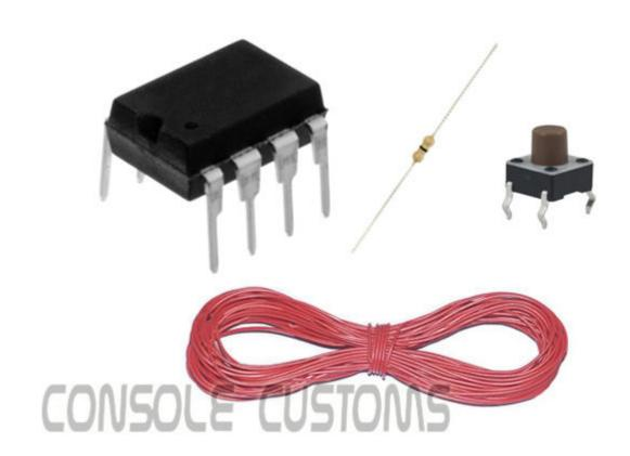
Step 1: You will start by taking the PIC chip and putting it on its back, also called (dead bug). Note the location of the notch that is on the top of the chip, the pin numbers and their purpose.
