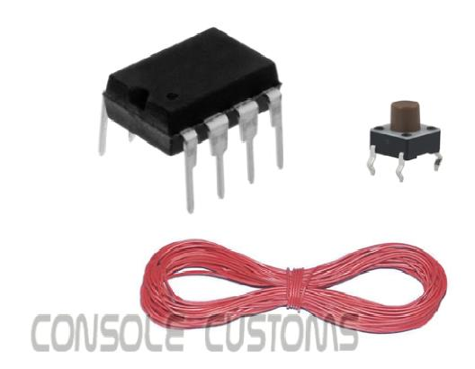
Step 2: You will start by taking the PIC chip and putting it on its back, also called (dead bug). Note the location of the notch that is on the top of the chip, the pin numbers and their purpose.
